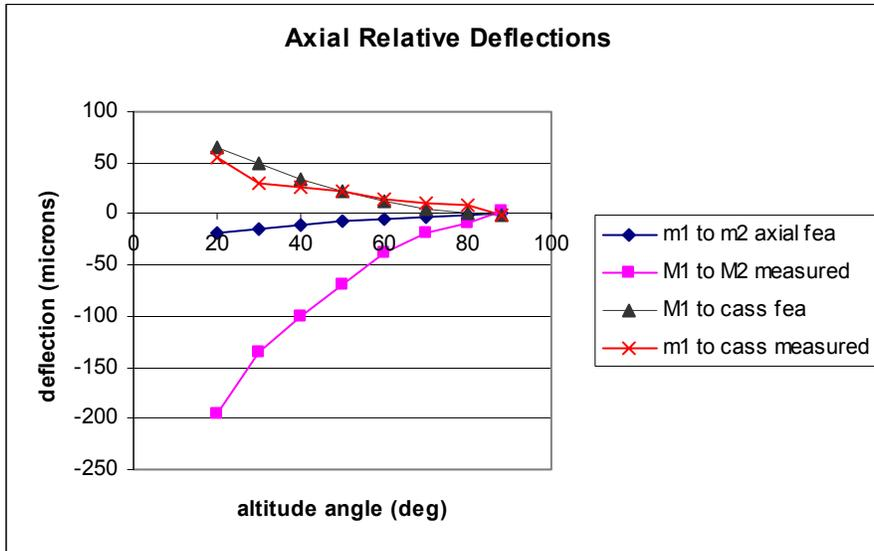
Figure 11 : Axial deflections FEA vs. Test
