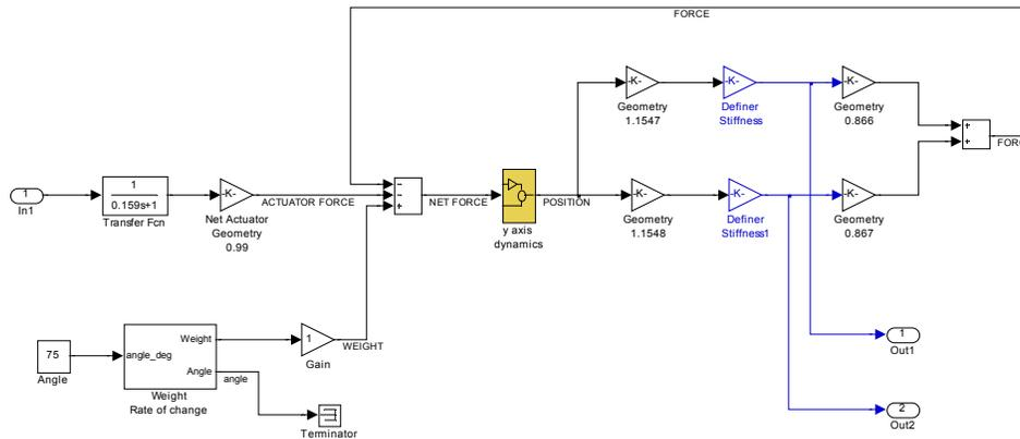
Figure 9 : Simulation for M1 Lateral Dynamics
