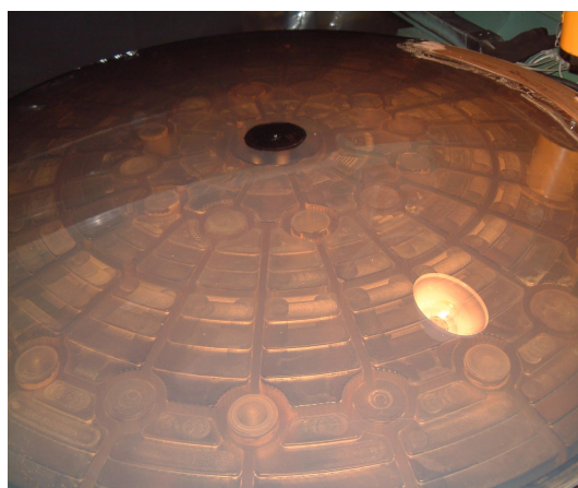
Figure 6: M2 showing lightweighting
