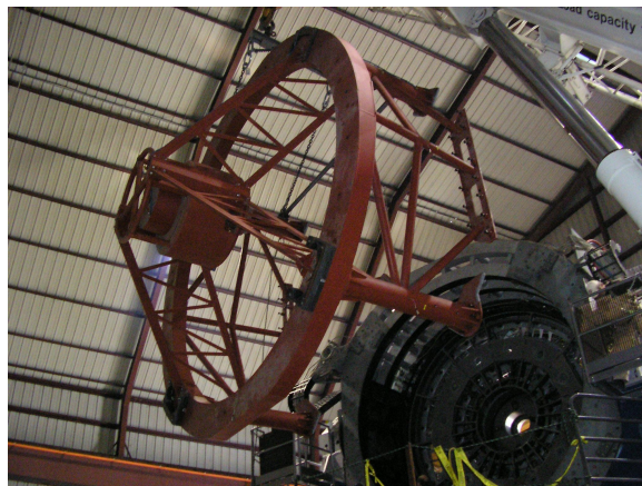
Figure 1 – Removal of the top end structure in preparation for M1 removal.
